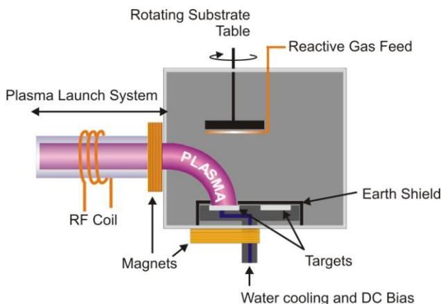
**Figure 1. A schematic showing the HiTUS system**
