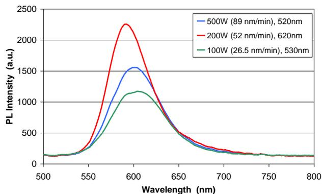
Figure 3. Variation of PL with target power
