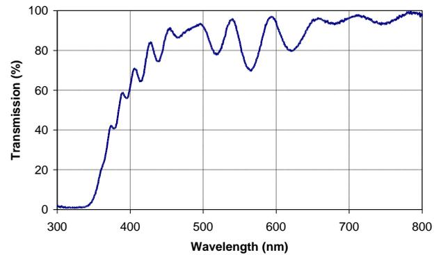
**Figure 6. Transmission profile of a complete EL device with ITO-Y<sub>2</sub>O<sub>3</sub>-ZnS:Mn-Y<sub>2</sub>O<sub>3</sub>-ITO structure.**
