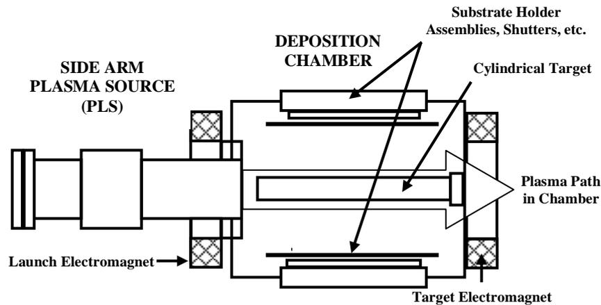
**Figure 2: 'Linear' System Layout (ILH550)**
